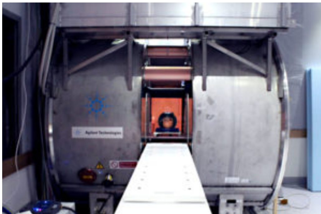
MRI Linac, a powerful experimental cancer radiation therapy system based at Liverpool Hospital
