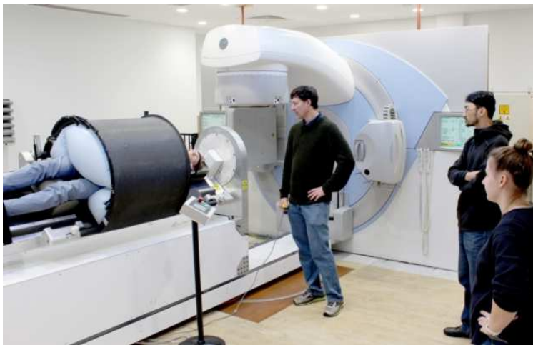
The prototype radiotherapy system combines a fixed vertical radiation beam with horizontal patient rotation. (Courtesy: Paul Liu)
